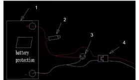
Fig 5. Electrical diagram of the battery box
