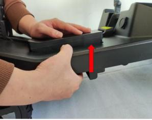
Fig 9. Battery box removal
