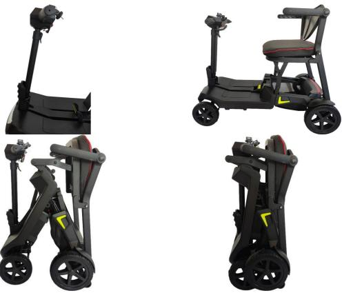
Fig 10. Disposition steps of scooter
