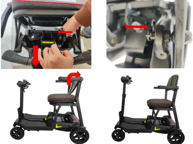
Fig 11. Steps of installing the scooter
